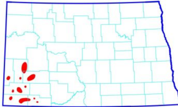
Known areas of uranium occurrence within 200 feet of the surface in western North Dakota. This information was plotted from radioactive spikes on gamma logs on file with the North Dakota Geological Survey.
